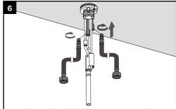
From the under-side of counter, screw the flexible hoses into the mixer body and fully hand tighten.
