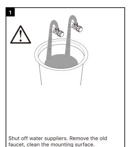
Note: For first time install, flush the pipes first by open the angel valve to run 60s.
