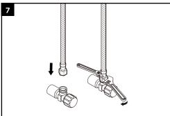
Connect and tighten the supply hoses by using two adjustable wrenches (avoid twisting or kinking).
