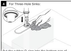
Put the rubber O-ring into the bottom gap of faucets then Insert faucet into faucet hole.
