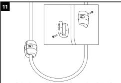
Install the hose weight on the outlet side of the hose, near the loop.
