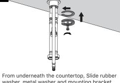
washer, metal washer and mounting bracket onto the thread shank.
