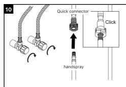
Shut off water suppliers. Push the handspray hose into the quick connector until you hear a click sound. Make sure it's secured.
