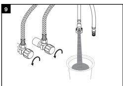
Turn on water suppliers. Place a bucket below outlet tube, slowly open and close the supply angle valves, This will prevent debris from being lodged in the hose and sprayer.
