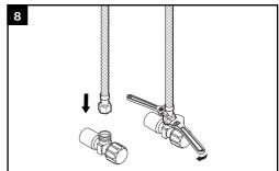
Connect and tighten the supply hoses by using two adjustable wrenches (avoid twisting or kinking).
