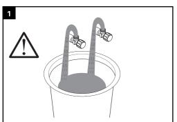
Shut off water suppliers. Remove the old faucet, clean the mounting surface.
