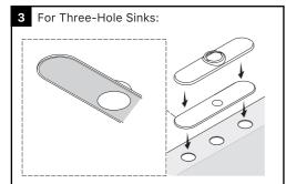
Place stainless (non-staining) deck plate and deck plate gasket onto sink, secure it with silicone. Note: the deck plate need purchase seprately.
