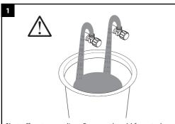
Note: For first time install, flush the pipes first by open the angel valve to run 60s.
