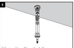
Adjust position of faucet body if necessary, Then tighten the mounting nuts with phillips screwdriver until snug.
