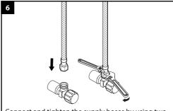
Connect and tighten the supply hoses by using two adjustable wrenches (avoid twisting or kinking).
