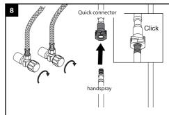
Shut off water suppliers. Push the handspray hose into the quick connector until you hear a click sound. Make sure it's secured.
