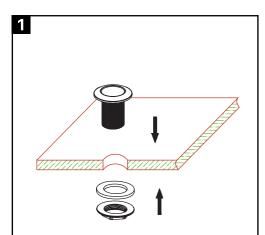
Put one washer into the groove in the bottom of the neck and then pass the threaded part of the neck through the countertop hole.
