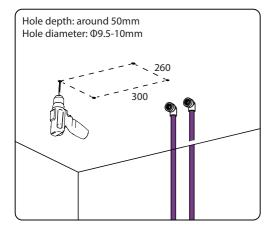
Use the bracket frame as temperate, marking the installation line by pencil. Drill 9.5-10mm diameter hole, depth around 50mm, then knock in the screw plug.
