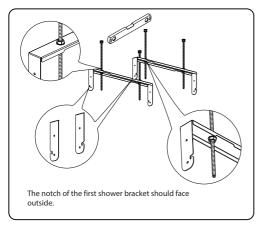
Install the shower bracket, make sure the brackets are at the same level, then tight the screw by spanner. Depending on different ceiling, the M6 expansion rod can be cut if necessary.
