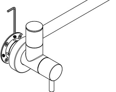
Once the faucet is level, use the provided Allen key to secure the flange and faucet in place.
