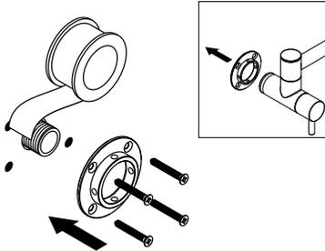
Wrap PTFE tape around the nipple, then secure the flange to the wall using screws.
