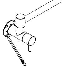
Rotate the flange to avoid pipes behind the wall, then mark the positions for the installation holes accordingly. Remove the faucet and flange from the wall, then drill holes at the marked positions. (Be careful of the pipes behind the wall.)
