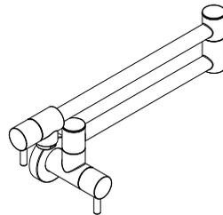
Remove aerator and turn faucet handles to the full on position. Turn on cold water supplies and flush water lines for one minute, check for leaks and proper operation.
