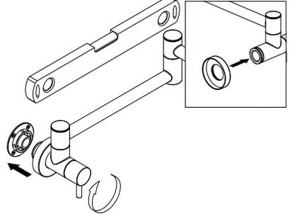
Install the faucet onto the nipple and use a small level to ensure it is straight.
