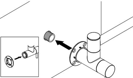
After attaching the flange to the faucet, install the faucet onto the 1/2 NPT nipple protruding from the wall. Do not over-tighten.
